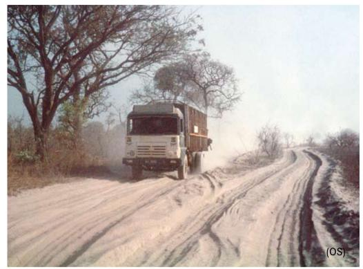
A truck driving over a temporary road on a terrace of the Volta River in Ghana creates huge dust clouds. This is due to the lack of cohesion between the particles in the topsoil.
