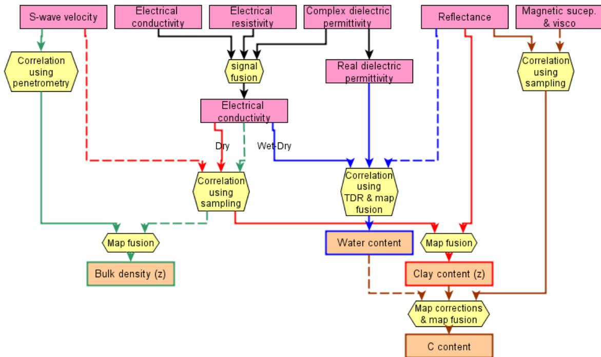
Figure 4 : Data assimilation from geophysical parameters to soil properties (from D2.1).
