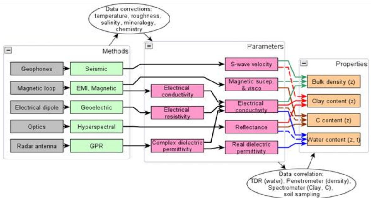
Figure 3 : Concept diagram showing the different paths for going from sensors to soil properties(from D2.1).
