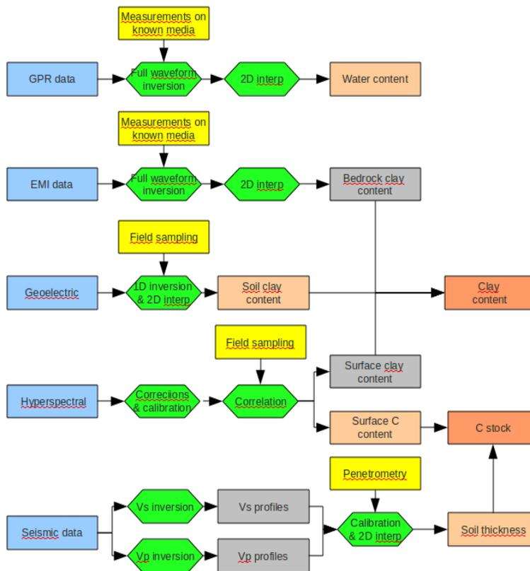
Figure 5 : Revised workflow of the Digisoil's system for estimating soil properties maps(from D3.3)
