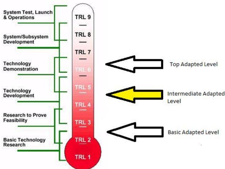
Figure 8 : The intermediate assessment level is identified as TRL levels four and five.
