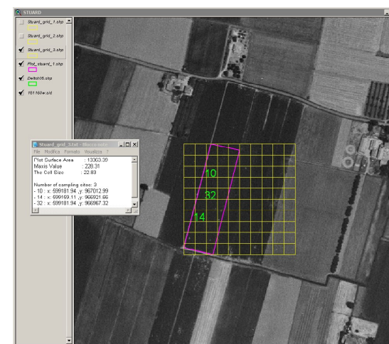
Automatic positioning and definition of the geographical coordinates of samples within an Area-Frame Randomized template for an agricultural location in Italy.
