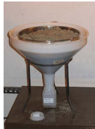
Figure 1—Berlese-Tullgren funnel, used for the soil microarthropods extraction
