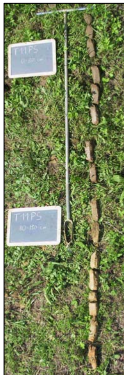
Figure 26. Drilling (site of the level II network)
