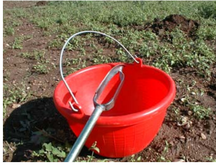
Figure 3. Particular of a manual drill for the collection of soil samples
