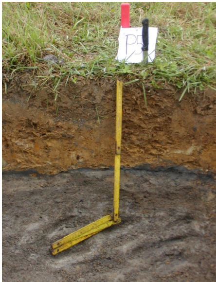
Figure 5: Covering of fly ash disposal by soil - combating the fly ash (orig.)
