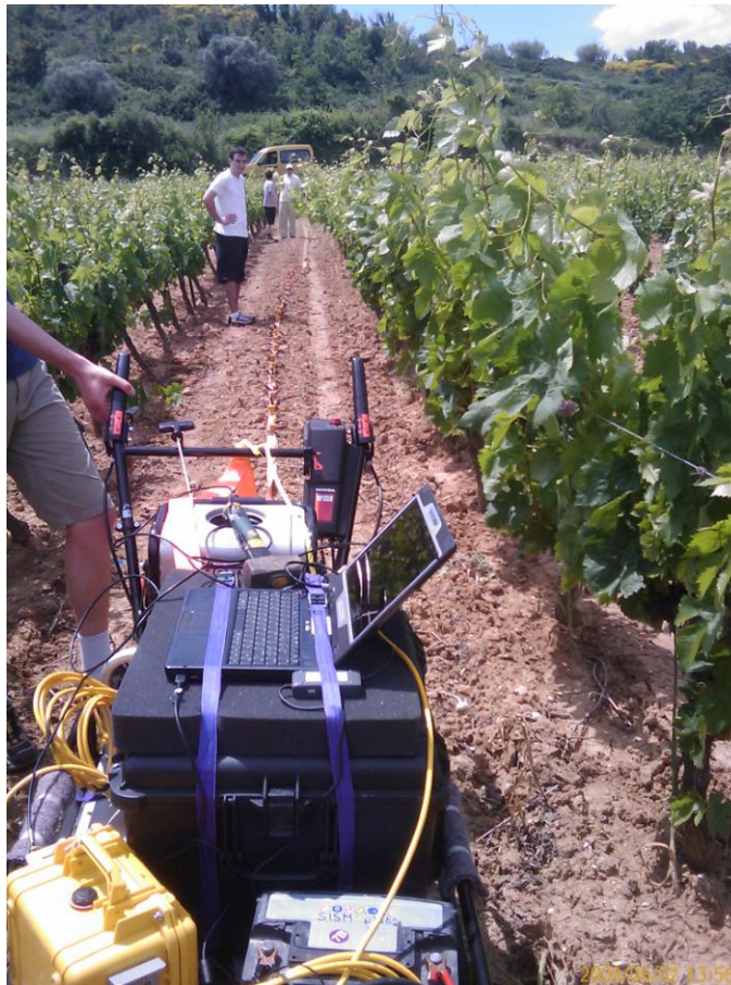
Figure 5 : Seismic device mounted on caterpillar-type vehicle for mapping of the soil shear waves velocity. The sensor system is mounted at the back of the vehicle. A computer automatically controls the measurements.
