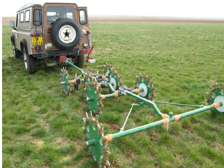
Figure 1: The MUCEP system: The data acquisition station is located inside the vehicle; The first two wheels carry the injection electrodes while 3 the last pairs carry measurements channels for 3 different spacings
