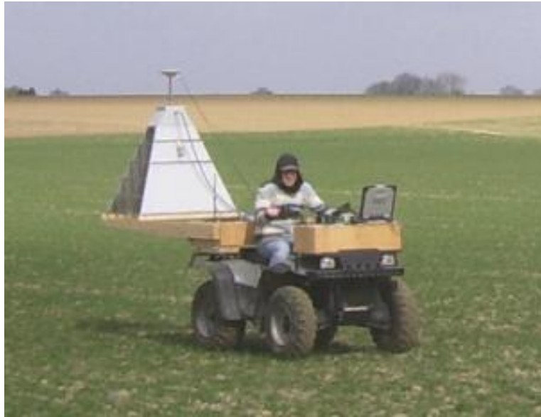
Figure 3: VNA ZVL from Rohde & Schwarz → SFCW radar, double ridged horn antenna BBHA 9120F from Schwarzbeck (Antenna dimensions : 96 x 68 x 95 cm and frequency range : 200-2000 MHz) The mode of operation is zero-offset, at 1.1 m above the ground.
