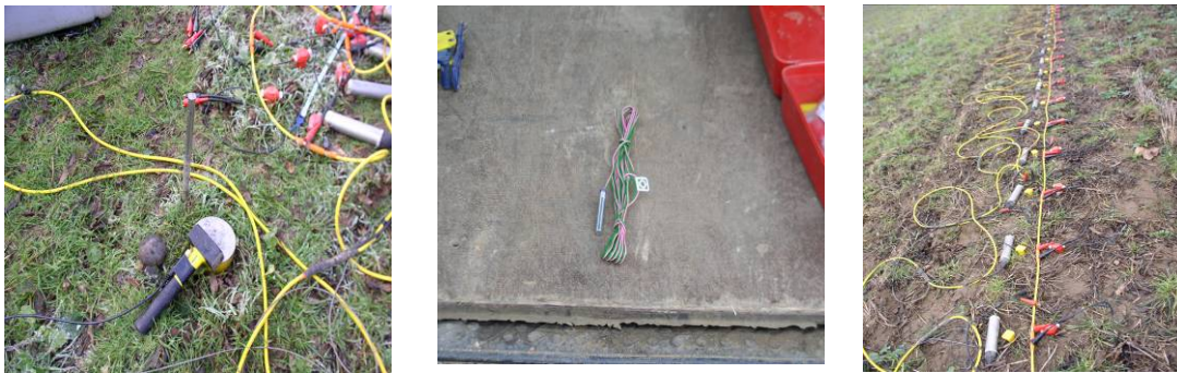
Figure 29: Tested seismic sources and receivers.
