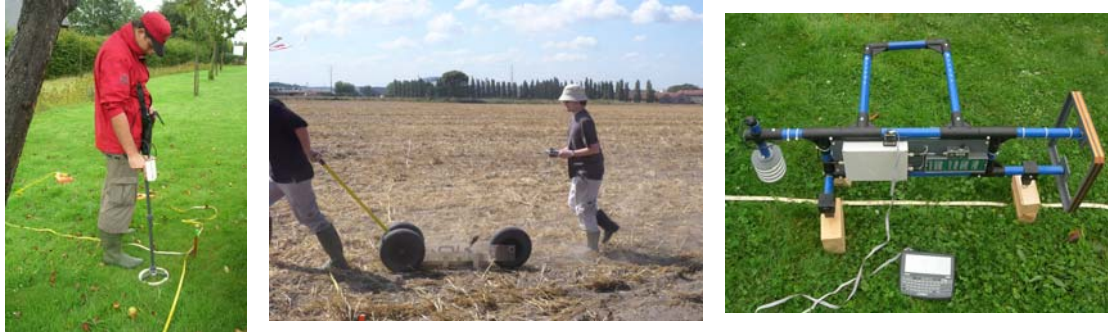
Figure 20: The chosen devices measuring the magnetic properties of soils (a) MS2D, Bartington Ltd; (b) CS60 on his carriage; (c) VC100
