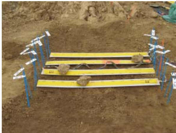
Figure 16: specific electrodes used for the characterisation of the soil structure at short scale. -a- plastic pan with electric electrodes spaced 10 cm apart. -b- Two plastic pans of 12 electrodes for a 24 Wenner array. -c- Four plastic pans of 12 electrodes for a 48 square array.
