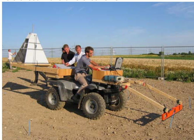
Figure 13 : EM38 mounted in front of a quad for real-time mapping of the soil electrical conductivity (Selhausen test site of FZJ). A GPR system is mounted at the back of the quad. A computer automatically controls the measurements.
