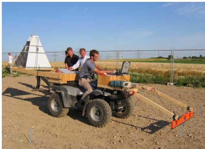
Figure 6 : GPR prototype mounted on quad for real-time mapping of the soil dielectric permittivity (Selhausen test site of FZJ).
