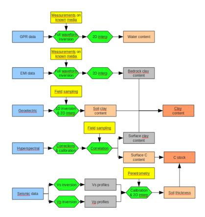
Figure 5 : Revised workflow of the Digisoil's system for estimating soil properties maps(from D3.3)
