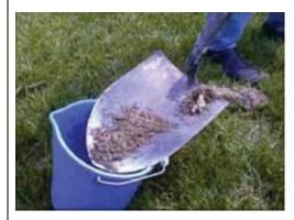
Put the soil in the bucket. Clean soil in excess from the spade.
