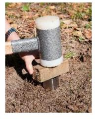
Excavate a little bit around the outside edge of the ring with a small, flat-bladed knife. Put the plastic cap to the ring.
