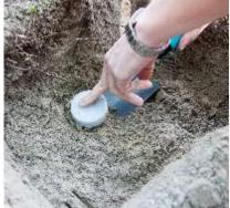
Remove excess soil from the bottom of the ring and around the outside edge of the ring with the knife.
