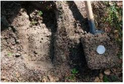
Remove excess soil from the bottom of the ring and around the outside edge of the ring with the knife.
