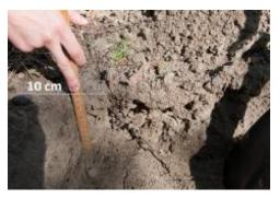
Gently press the metallic ring, bevelled edge down, into the soil with the help of a mallet. Use a block of wood to push the ring with the mallet, in order to avoid compaction of soil and protect the ring. Avoid pushing the ring in too far or the soil will compact.
