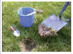
Remove vegetation residues, grass and litter, if any, from the surface. Some fine roots and brownish organic material from the upper part of the soil can remain in the sample, as it is difficult to remove it completely.
